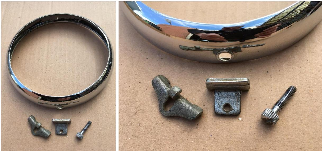
*Some head light rims were of a type with a bottom hole, which needed different mounting materials like the catching bracket as shown in the image above.*
